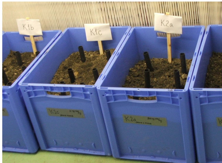
Figure 2: The second approach set-up. Perforated pipes constitute the aeration system due to convection.
