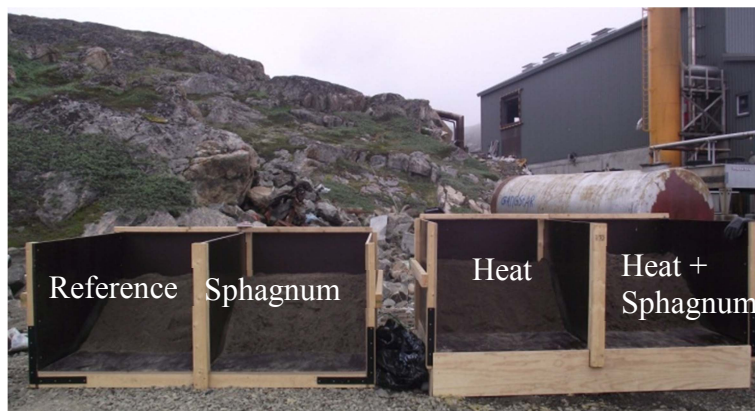
Figure 3: Boxes with oil-contaminated soil and different additions. The addition of sphagnum includes both sphagnum moss and chalk.
