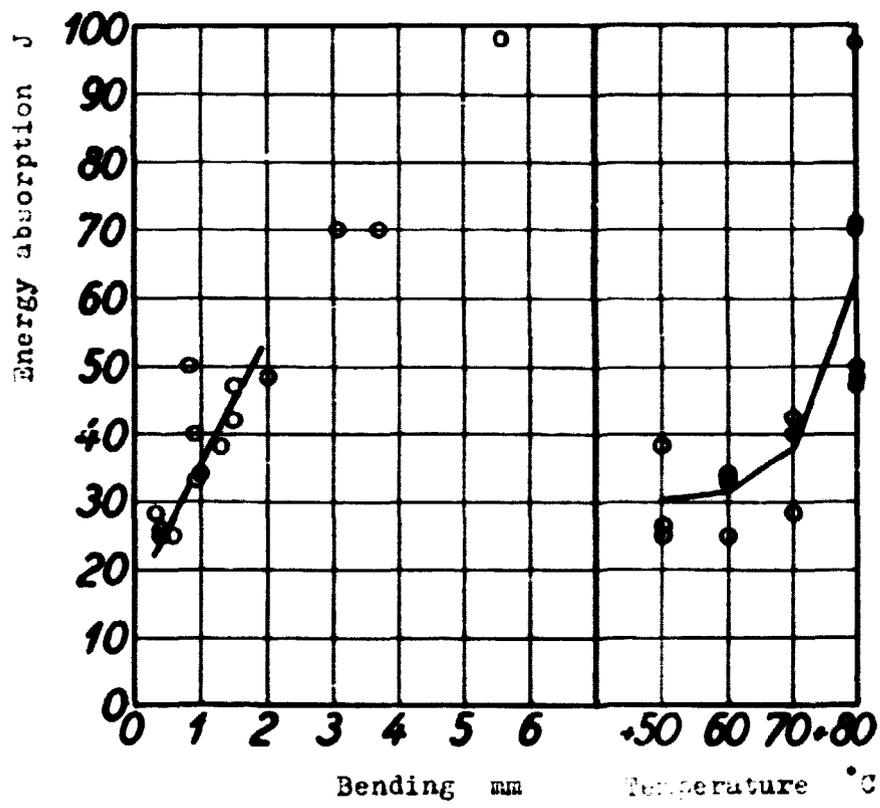
Fig. 6. Steel 2253. Charpy-C testing.
