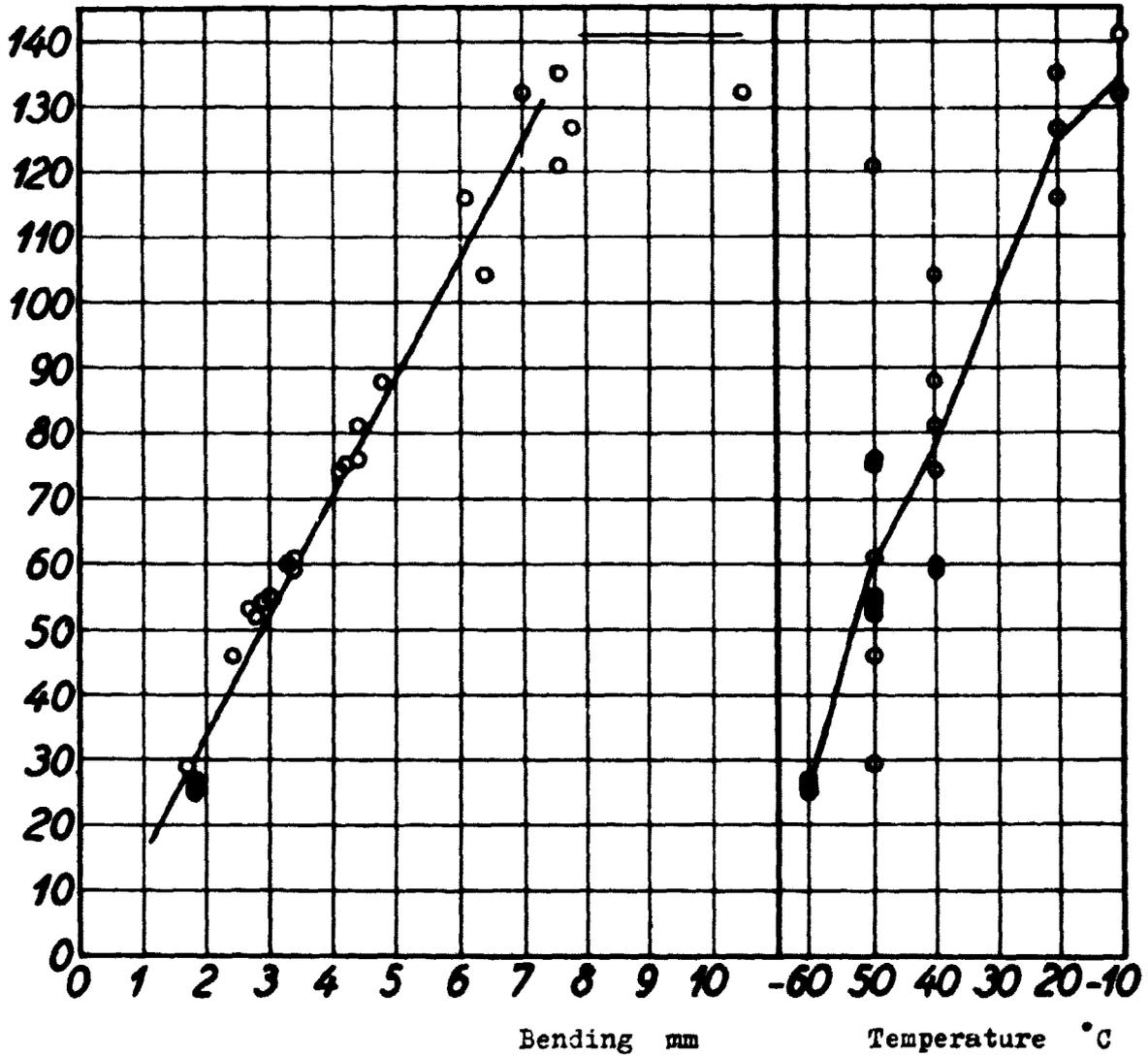
Fig. 4. Steel 2251. Charpy V-notch testing.
