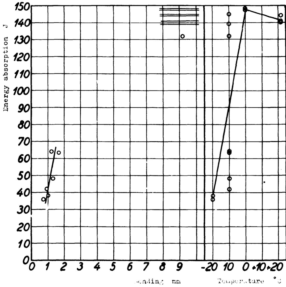
Fig. 7. Steel 2251. Charpy-C testing.
