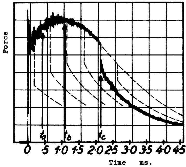
Fig. 2. Diagram recorded during Charpy V-notch testing.
