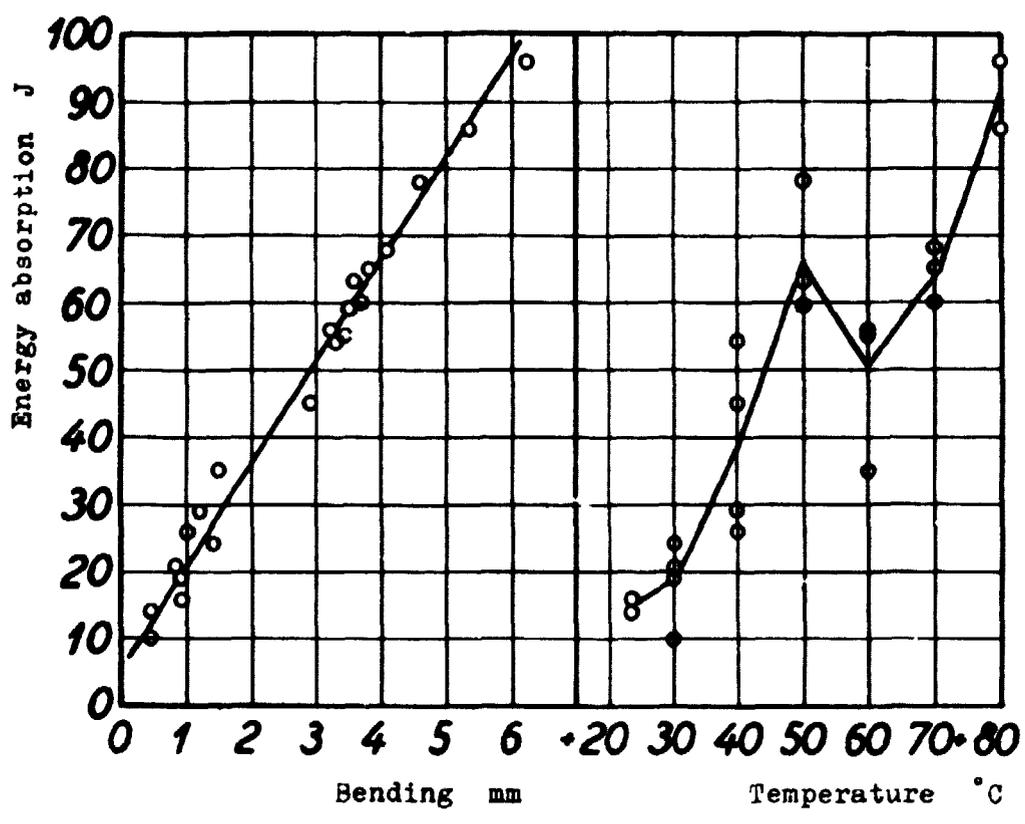
Fig. 3. Steel 2253. Charpy V-notch testing.
