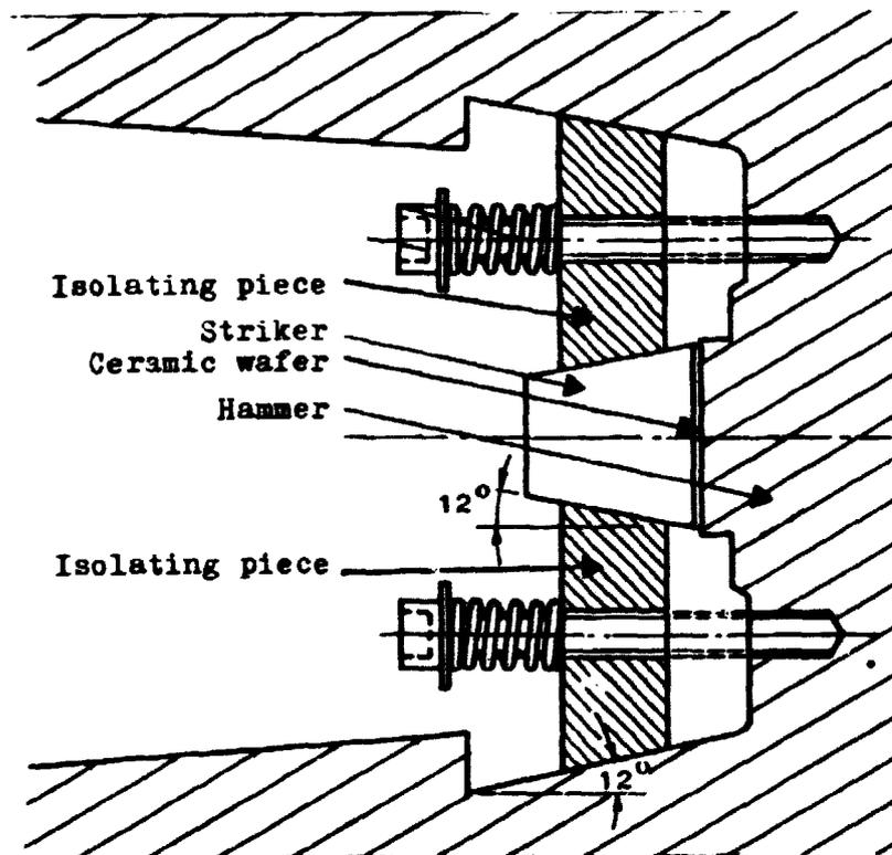
Fig. 1. Pressure transducer.
