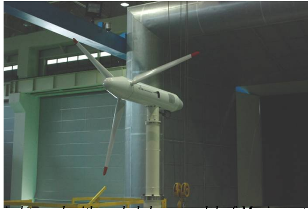
Figure 10.1 KARI wind tunnel with scaled down model of Mexico rotor, compare with figure 4.2
