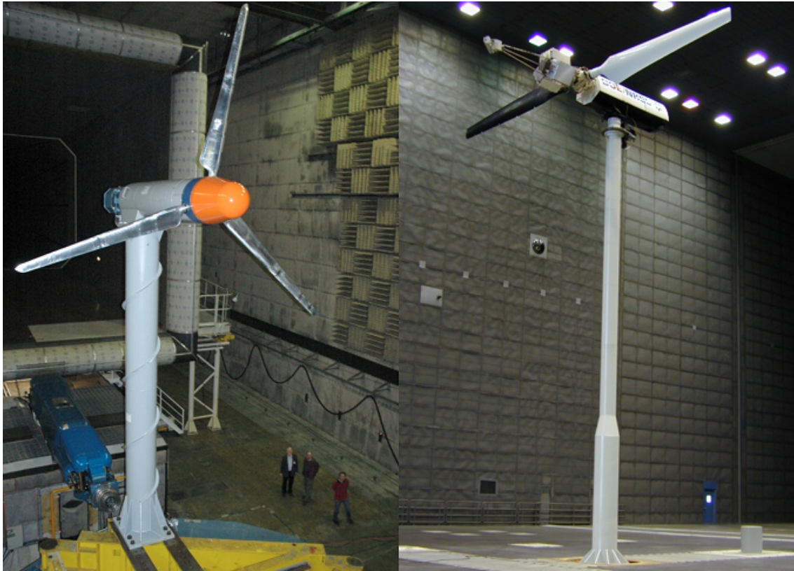
Figure 15.7 MEXICO turbine in the DNW LLF 9.5 m x 9.5 m open jet (left), and the UAE Phase VI turbine in NASA Ames 24.4 m x 36.6 m wind tunnel (right).
