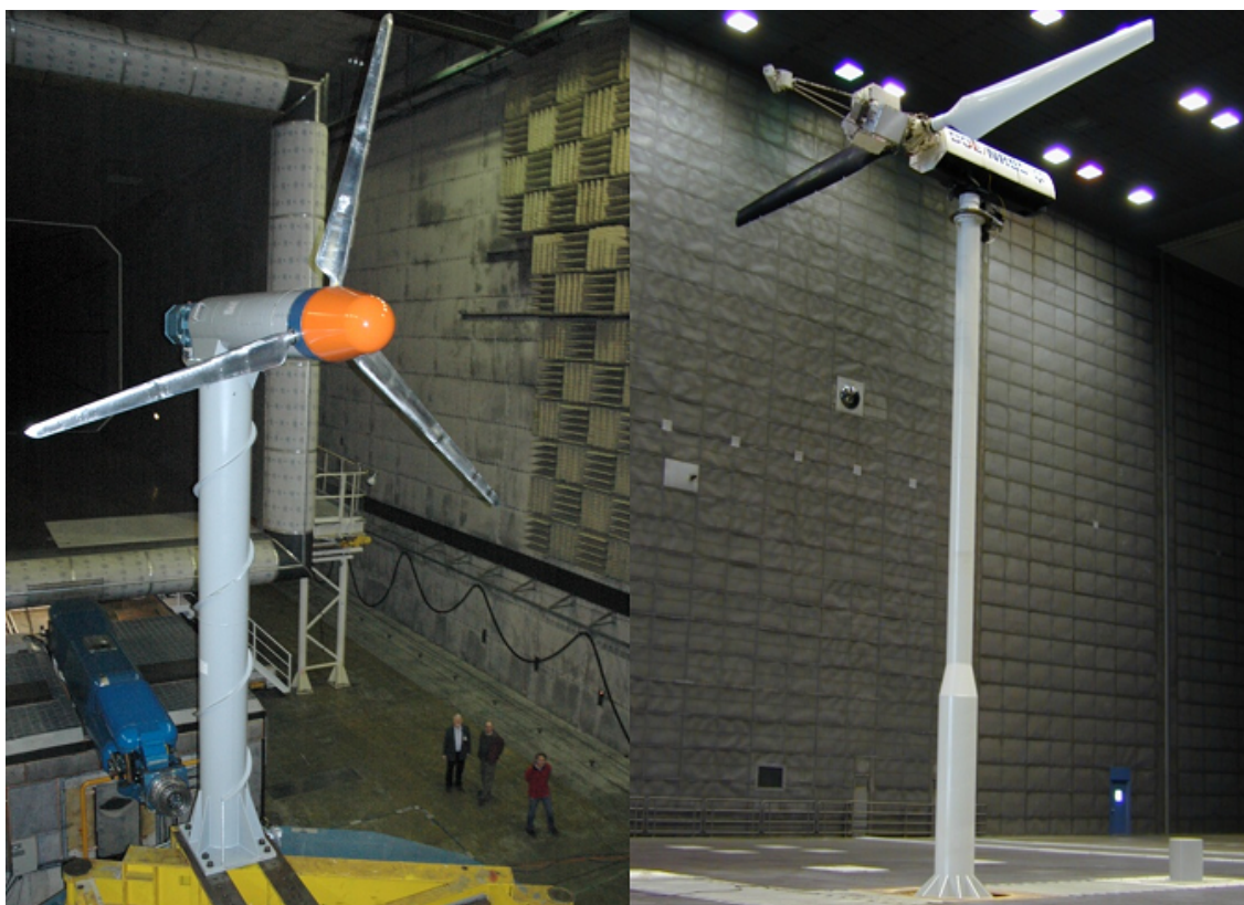
Figure 15.7 MEXICO turbine in the DNW LLF 9.5 m x 9.5 m open jet (left), and the UAE Phase VI turbine in NASA Ames 24.4 m x 36.6 m wind tunnel (right).
