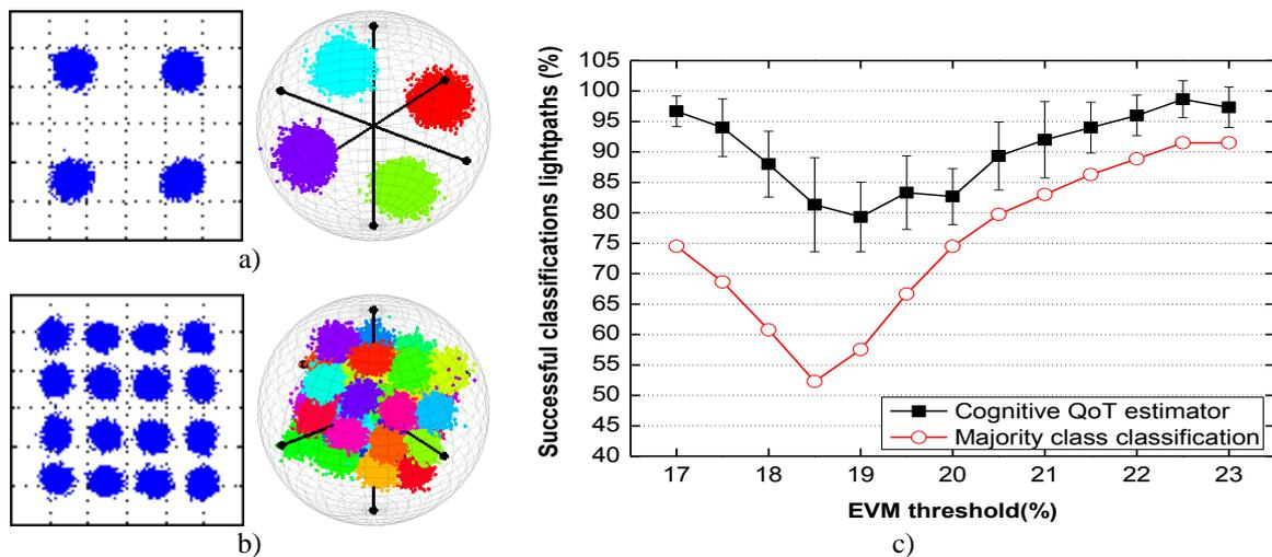
Figure 3. Modulation format recognition in Stokes space, experimental results for a) DP-QPSK b) DP-16QAM c) Experimental demonstration of QoT based on CBR for PD-QPSK WDM networks with high successful ratio for small KB [13].
