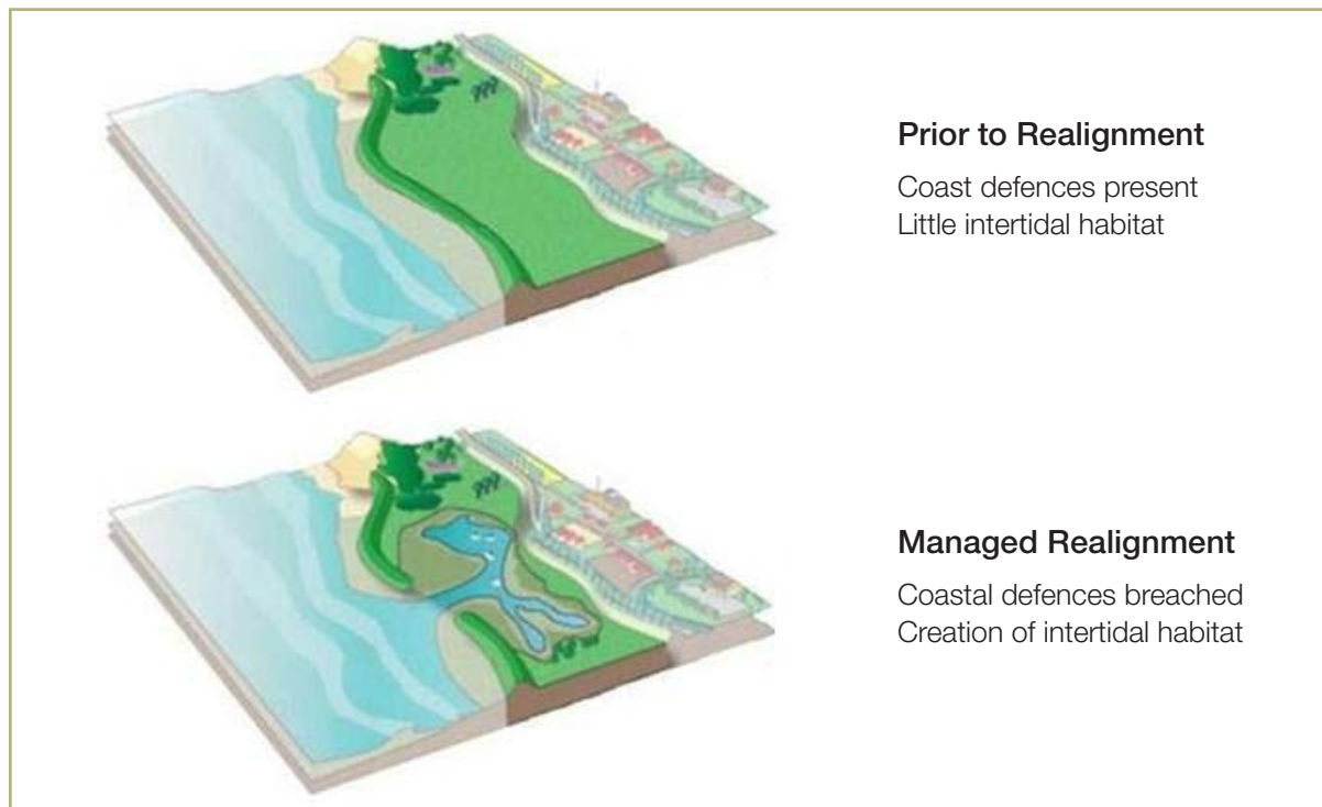
Figure 4.28: The process of managed realignment
