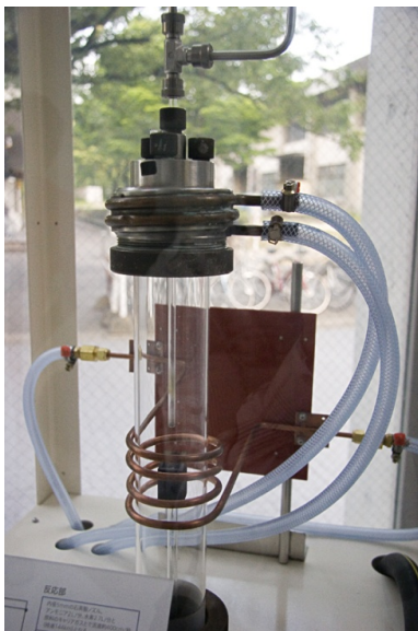
Figure 1. (a) A replica of MOVPE equipment to demonstrate buffer layer technology and high gallium nitride crystal quality; (b) One of the MOCVD equipments that were used to achieve magnesium doping.
