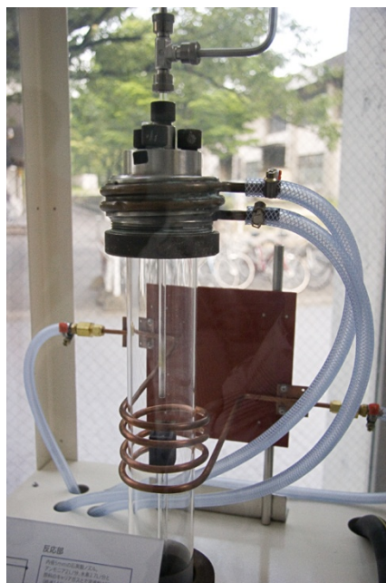
Figure 5. A replica of the reactor used by Akasaki to develop the growth technology for gallium nitride used for blue and white LEDs.
