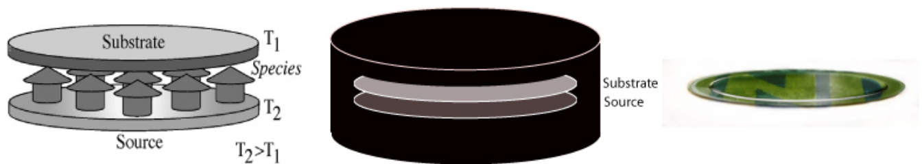
Figure 7. The configuration for the Fast Sublimation Growth Process.
