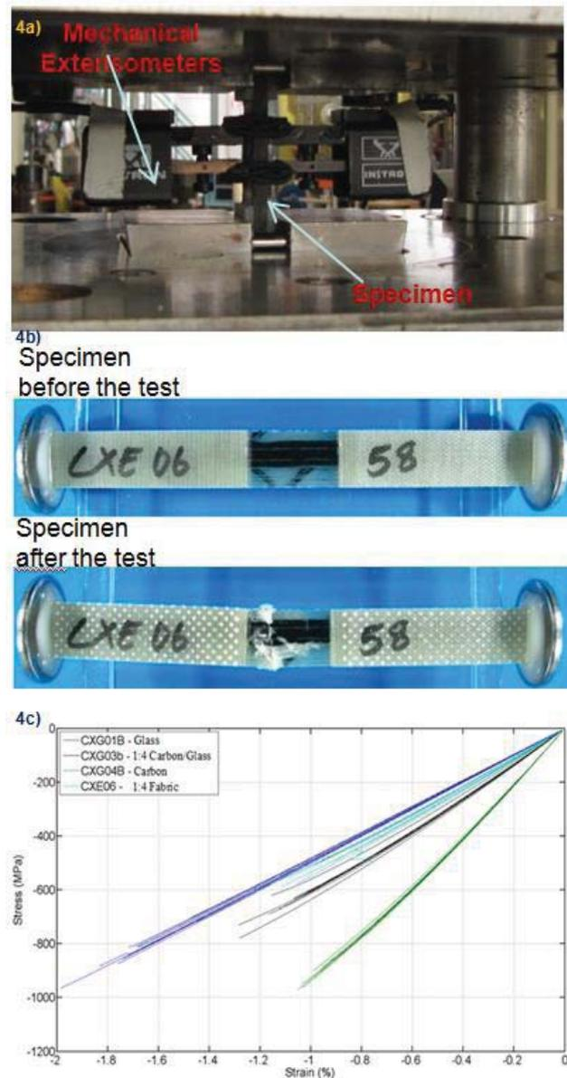
Figure 4.a. Test specimen fixed in the MCL fixture.
