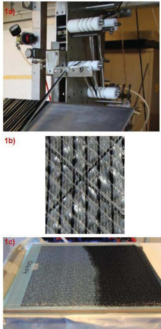
Figure 1. a. Filament winding setup
