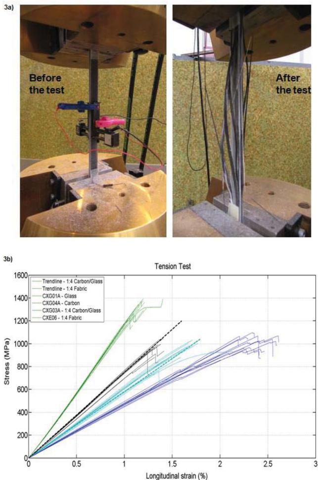
Figure 3. a. Tensile test setup with mechanical extensometers and specimen, before and after test
