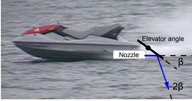
Fig. 1. PWC with deflected elevator: a deflection \beta causes the water jet to be deflected by an angle equal to 2\beta .
