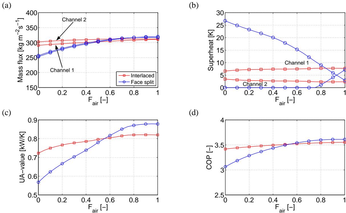
Figure 4. Selected parameters vs. the airflow distribution parameter
