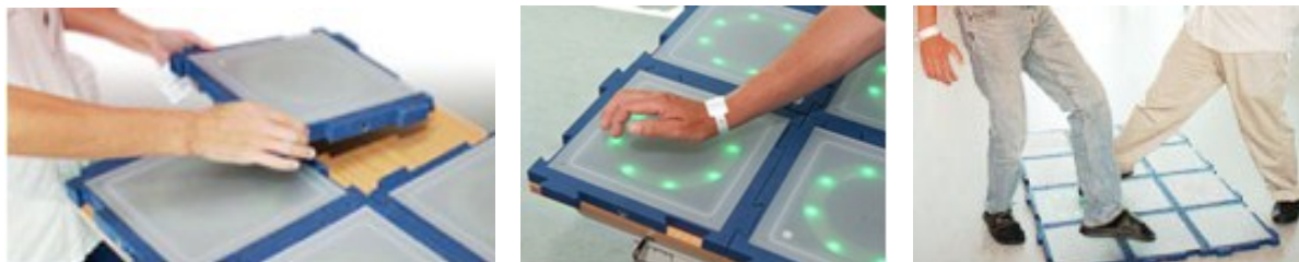
Figure 1. Modular tiles assembled and used for hand or feet interaction.
