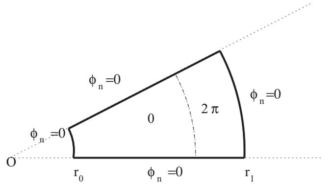
FIG. 1. Sketch of the 2D domain for the sine-Gordon equation. The radial kink initial condition is shown as a dotted-dashed line.
