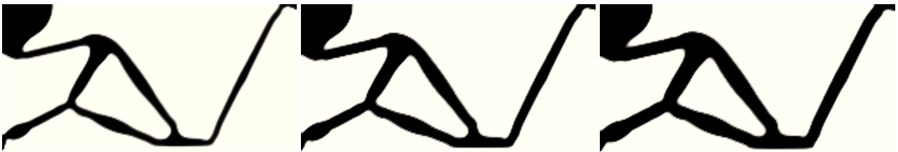
Figure 5. Three threshold projections, eroded, intermediate and dilated, obtained with thresholds \eta = 0.6, 0.5 and \eta = 0.4 , respectively. The design is obtained using large displacements robust optimisation formulation with threshold \eta \in \mathcal{U}[0.3, 0.7] and volume constraint 30% of the original volume imposed on the dilated projection at \eta = 0.3 . The objective is E[c] = -8.96 \mu\text{m} , the standard deviation is STD[c] = 5.80 , the number of the integration points is 31, and the projection parameter is \beta = 32 .
