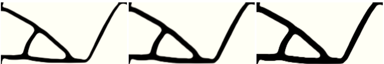
Figure 6. Three threshold projections, eroded, intermediate and dilated, obtained with thresholds \eta = 0.6, 0.5 and \eta = 0.4 , respectively. The design is obtained using large displacements robust optimisation formulation with threshold \eta \in \mathcal{U}[0.2, 0.8] and volume constraint 30% of the original volume imposed on the dilated projection at \eta = 0.2 . The objective is E[c] = -6.12 \mu\text{m} , the standard deviation is STD[c] = 4.00 , the number of the integration points is 31, and the projection parameter is \beta = 32 .
