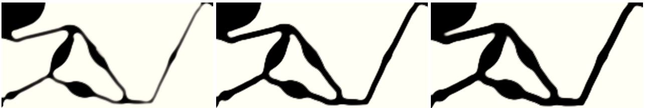
Figure 4. Three threshold projections, eroded, intermediate and dilated, obtained with thresholds \eta = 0.6, 0.5 and \eta = 0.4 , respectively. The design is obtained using large displacements robust optimisation formulation with threshold \eta \in \mathcal{U}[0.3, 0.7] and volume constraint 30% of the original volume imposed on the dilated projection at \eta = 0.3 . The objective is E[c] = -7.85 \mu\text{m} , the standard deviation is STD[c] = 1.0 , the number of the integration points is 2, and the projection parameter is \beta = 32 . The objective expectation and standard deviation, computed with 31 integration points Kronrod-Patterson rule are E[c] = -8.43 and STD[c] = 5.83 .
