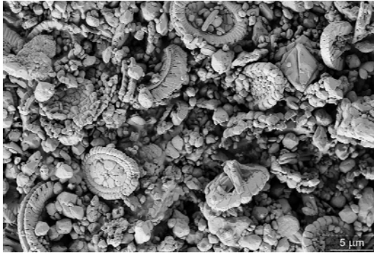
Figure 1: Scanning Electron Microscopic (SEM) image of chalk from Stevns (outcrop Denmark) showing pore spaces in between calcareous skeletons and skeleton fragments (Hjuler et al., 2007).
