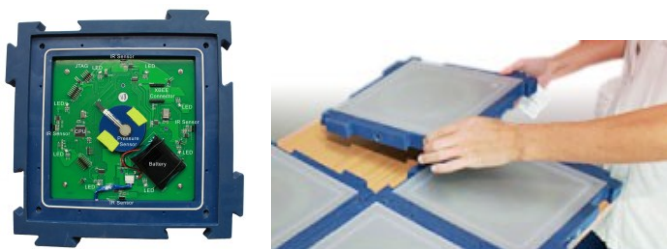
Figure 5. Left: PCB and components of a modular interactive tile. Right: Assembly of the modular interactive tiles as a simple jigsaw puzzle.
