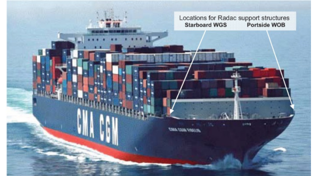
Fig. 1: Considered vessel and location of instantaneous wave height meters (Radac system).
