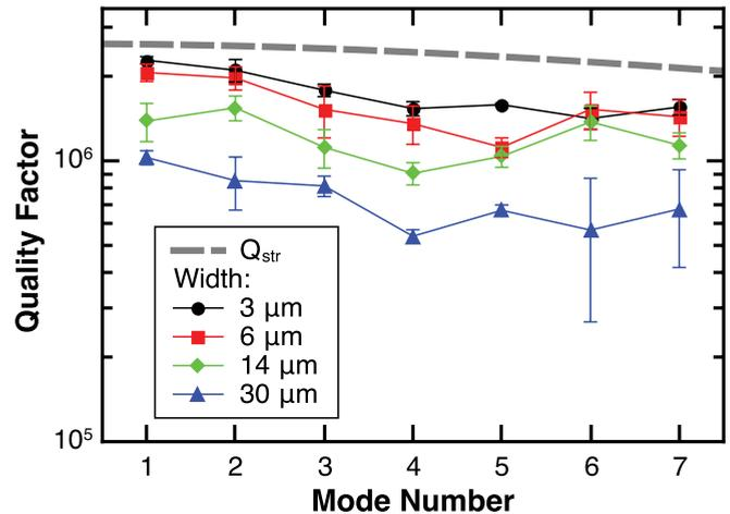
FIG. 5. (Color online) Quality factors of 1067- $\mu\text{m}$  long low-stress silicon nitride strings for higher bending modes for varying width. Every data point represents the average of three strings. The dashed line represents the calculated maximal quality factor due to intrinsic material damping  $Q_{\text{str}}$  (11).
