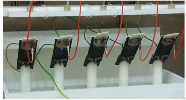
Fig.4 – Tracking resistance test setup. Set of 5 samples mounted on the supports.
