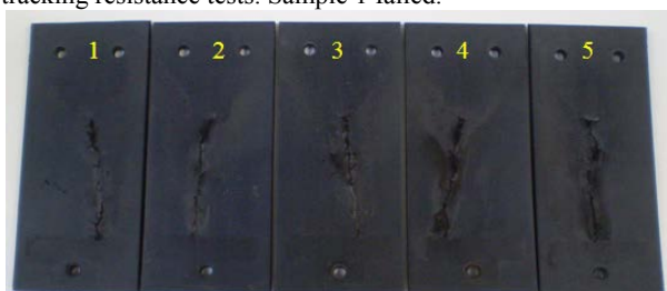
Fig.10 – Surface erosion in EPDM rubber material after the tracking resistance tests. All samples failed.
