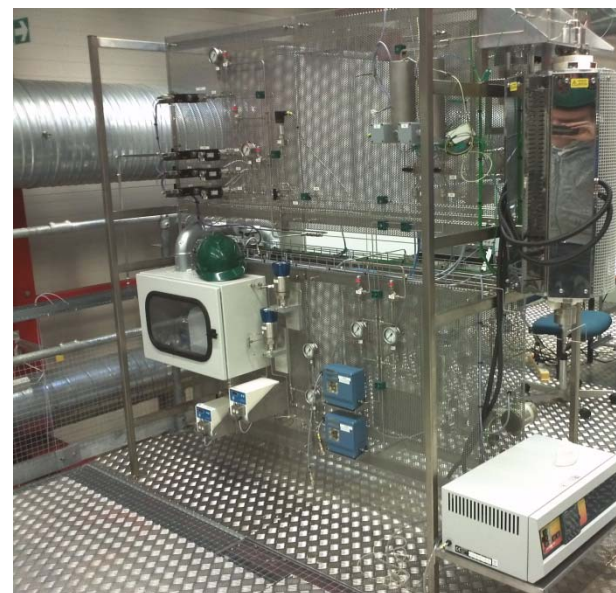
Study on catalysts for hydrodeoxygenation of pyrolysis oil – High pressure flow reactor, up to 125 bar and 550°C
