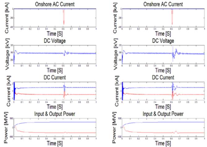
Figure 10: On the left *MMC response to dc link short circuit fault* a) AC phase voltage b) AC phase current c) DC link voltage for one pole d) DC current e) Active power transfer, on the right *MMC response to dc link short circuit fault with increased transformer series capacitance*.
