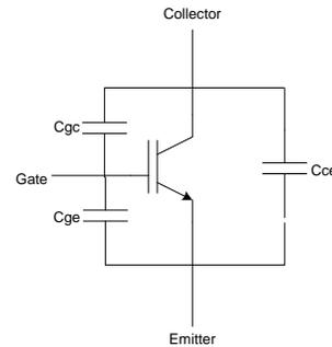
Figure 6: Capacitances of an IGBT [7]
