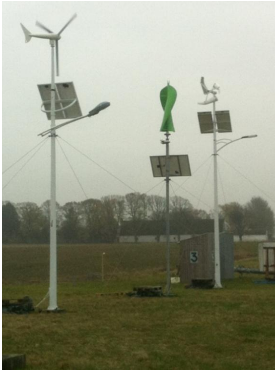
Figure 7: Picture of 3 hybrid lighting system masts - the two outer masts are equipped with data logging. The masts are numbered 1 to 3 from the right, so the right one is called number 1.
