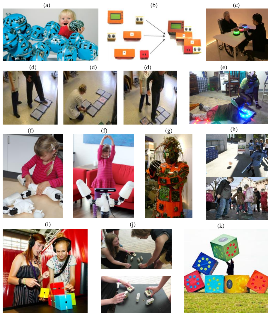
Fig. 1. Examples of modular systems with user interaction: (a) ATRON self-reconfigurable modular robot, (b) I-Blocks in LEGO Duplo, (c) Light&Sound Cylinders and Rolling Pins for elderly dementia patient therapy in multi-sensory room, (d) modular interactive tiles for rehabilitation of stroke and cardiac patients, (e) modular interactive tiles for rehabilitation of mentally and physically handicapped children in Africa, (f) Fable user-configurable modular robot, (g) Fatherboard modular robotic wearable, (h) modular interactive tiles for soccer and playgrounds, (i) Music I-Blocks, (j) MusicTiles magic matchboxes, (k) MusicTiles magic cubes.
