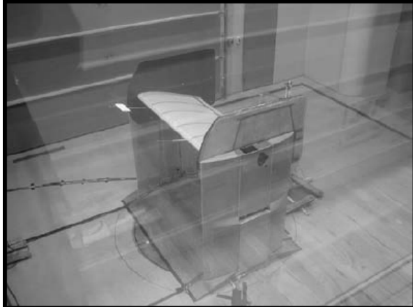
Figure 2. The wind tunnel model with a chord of 1 m and span of 1.9 m equipped with a 15% c CRTEF.
