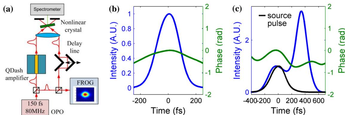
**Fig. 3 – (a) The X-FROG scheme. (b) Retrieved source pulse. Intensity is normalized so that the peak reaches unity. (c) Retrieved pulse after propagating through the amplifier. The source pulse is marked for comparison. Intensity is normalized so that the first peak reaches value of unity.**
