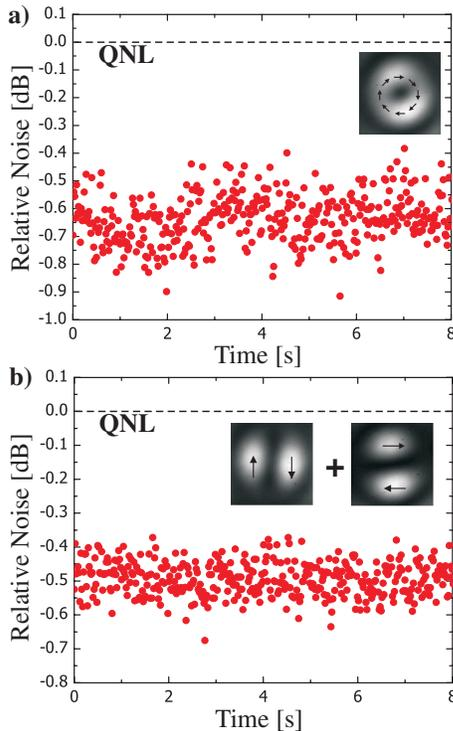
FIG. 4 (color online). (a) A quantum noise reduction of 0.6 dB is observed in the azimuthally polarized mode. (b) Anticorrelations of 0.5 dB below the QNL of the horizontally polarized  $TEM_{01}$  and vertically polarized  $TEM_{10}$  have been measured. The insets illustrate the measured spatial modes and the arrows indicate the polarization of the state.
