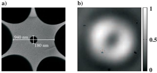
FIG. 2 (color online). (a) The specially designed photonic crystal fiber which supports the azimuthally polarized mode. (b) Normalized mode intensity profile of the azimuthally polarized mode at  $\lambda = 810$  nm, measured after the fiber.
