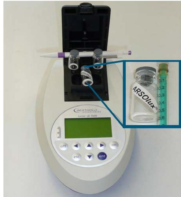
Figure 1. ARSOlux<sup>®</sup> glass vials containing freeze dried bioreporter bacteria and portable luminometer for arsenic measurement.
