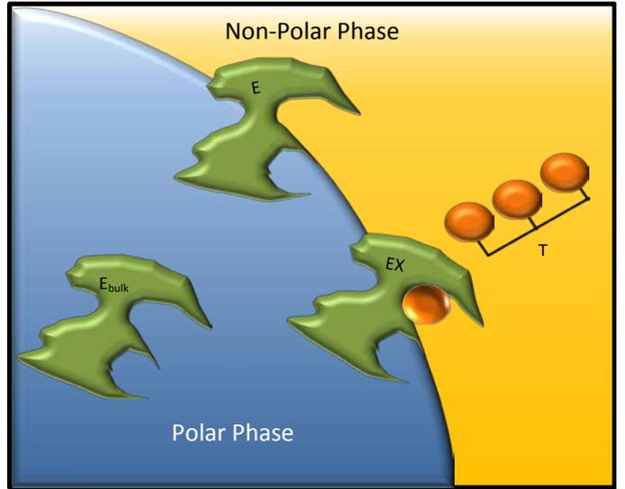
**Fig. 1. Diagrammatic representation of the enzyme at the oil water interface. The polar phase contains water, methanol, glycerol and the Free enzyme ( $E_{bulk}$ ). The non-Polar phase contains the oil components along with the biodiesel formed. At the interface is the penetrated enzyme ( $E$ ) and the Acyl Enzyme complex ( $EX$ )**
