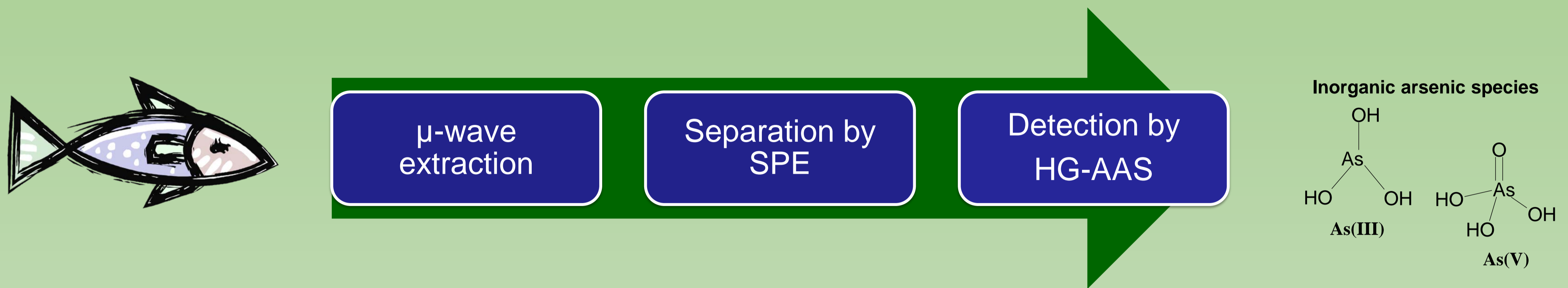
FIGURE 1. Principle of the MAE-SPE-HG-AAS approach for selective speciation analysis of inorganic arsenic.
