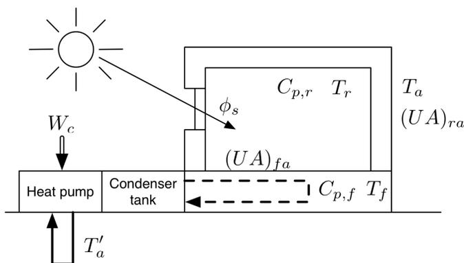
Fig. 1 House and heat pump floor heating system and its thermal properties. The dashed line represents the floor heating pipes. The term  $UA$  is a product of the heat conductivity and the surface area of the layer between two heat exchanging media. Its reciprocal value  $R = 1/(UA)$  is often used and is interpreted as a resistance against heat flow.  $C_p$  is the heat capacity and  $T_a$  is the ground temperature.
