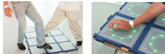
Fig. 1. Modular tiles used for feet or hand interaction.
