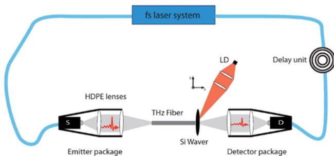
Fig. 1 Schematic of the THz near-field setup
