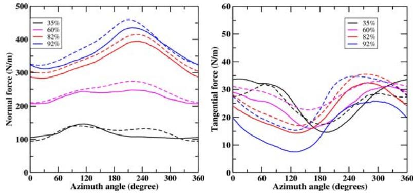
Figure 2: Comparison between computations and experimental data for flows past the MEXICO 25 kW rotor at a wind speed of 15 m/s and a yaw angle of  $45^\circ$  (solid line: experiment; dashed line: computation with MAD).
