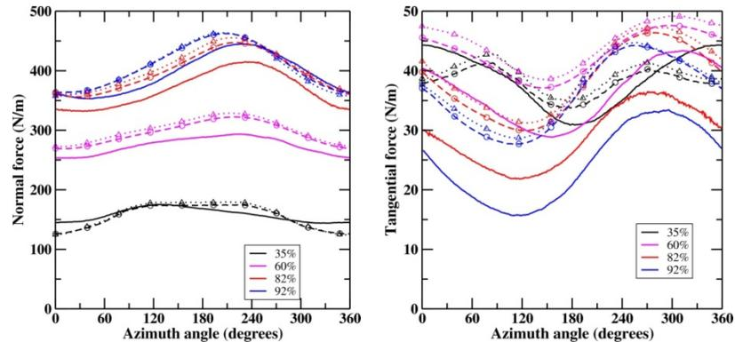
Figure 8: Comparison between computations and experimental data for flows past the MEXICO rotor at a wind speed of 15 m/s and a yaw angle of  $30^\circ$  (solid line: experiment; dashed line: computation with MAD in free air; dotted line: computation with MAD with tunnel).
