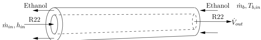
Figure 6.4: Sketch of test case evaporator
