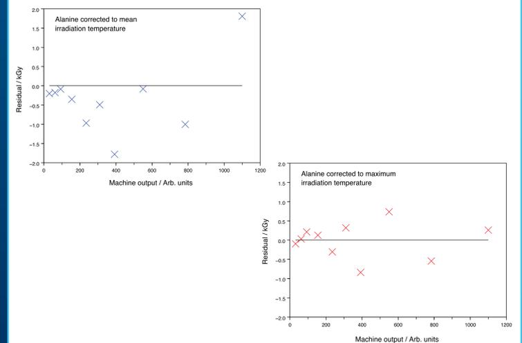
Figure 6. Residual plots of through origin first order regression fits of alanine dose as a function of machine output.
