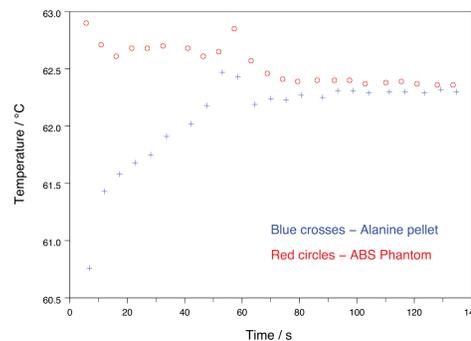
Figure 2. Temperature of alanine pellet and surrounding ABS phantom immediately after irradiation.
