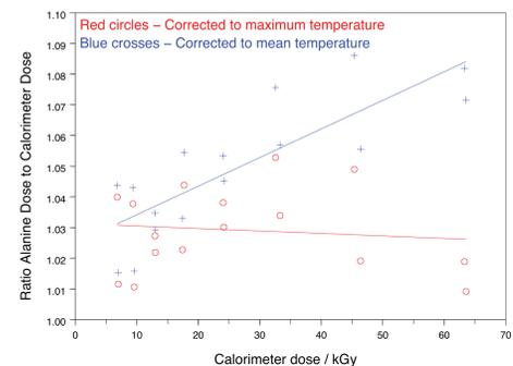
Figure 4. Ratio of alanine dose to calorimeter dose corrected to maximum and mean irradiation temperatures.
