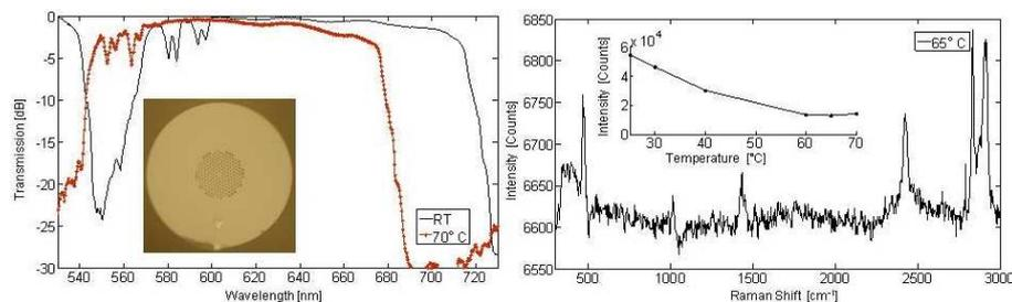
**Fig.1** (Left) Transmission spectra of the device at RT (22°C) and at 70°C, both normalized to the spectrum of the unfilled fiber; (Right) Raman spectrum of cyclohexane transmitted through the filled fiber, at 65°C. Inset: attenuation of the Rayleigh line due to the tuning of the filter.
