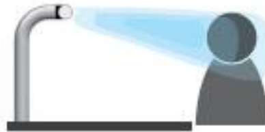
Figure 1: Typical set-up of personalized ventilation system.
