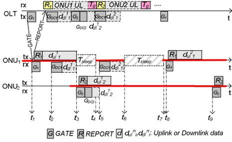
Fig. 2. EPON system with DCS energy management.
