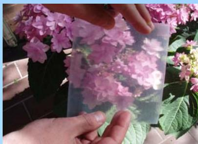
Fig. 3: PLA film with 2 % Hycite 713, thickness: 250 µm.
