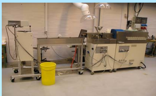
Fig. 1: Twin-screw extruder used for compounding.
