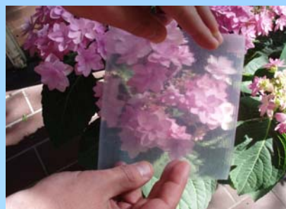
Fig. 3: PLA film with 2 % Hycite 713, thickness: 250 µm.
