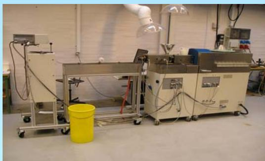
Fig. 1: Twin-screw extruder used for compounding.
