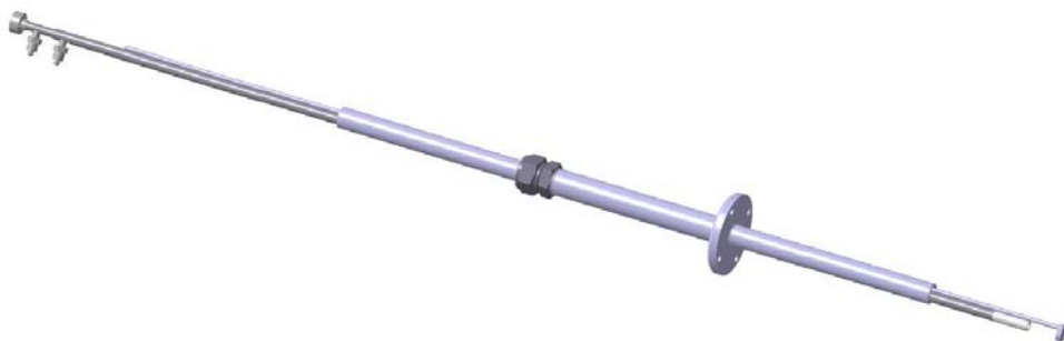
Figure 7 The water-cooled fiber-optic probe for measurements of gas temperature and gas composition in the laboratory scale oxy-fuel flame. The FTIR-probe is inserted into a port holder with flange for leak tightness and easy handling during experiments.
