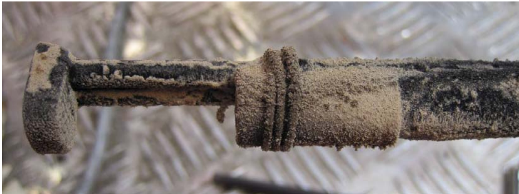
Figure 9 Deposits on FTIR-probe after measurements in the flame. The first layer on water-cooled stainless steel probe is soot (black areas). A simple wire supports the mounting of the ceramic tube on the probe. Optics is placed 20-30 mm inside the probe from the tip of the ceramic tube.
