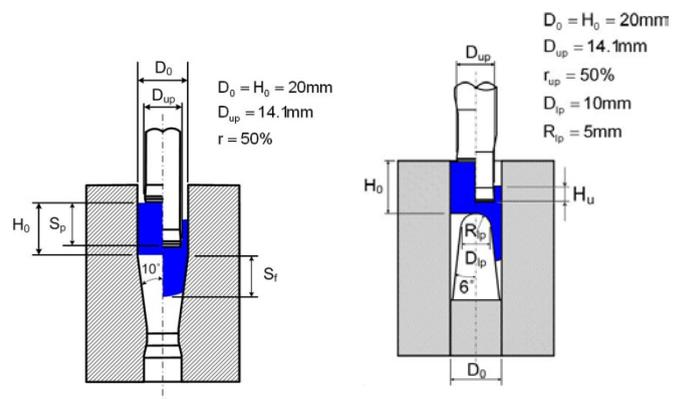
Figure 6. Lubricant testing by Forward-Rod/Backward-Cup [42]. Figure 7. Lubricant testing by Forward-Conical-Cup/Backward-Straight-Cup [43].
