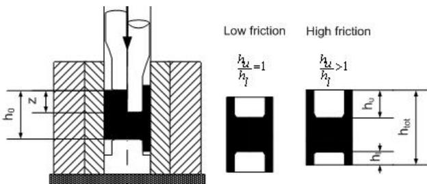
Figure 13. Schematic outline of double cup extrusion test.
