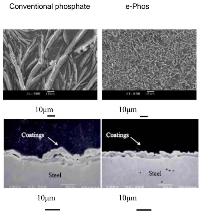
Figure 1. SEM and LOM micrographs of conventional and electrolytic phosphate coatings [24].
