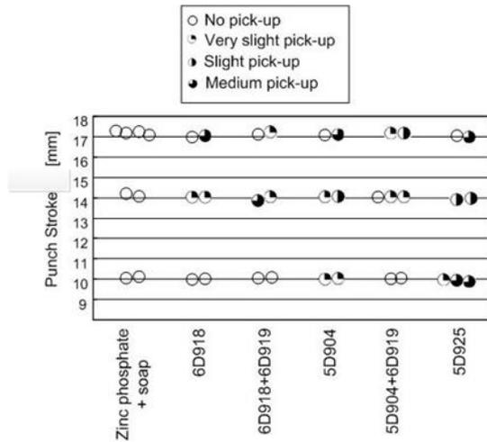
Figure 8. Limits of lubrication in Forward-Conical-Cup/Backward-Straight-Cup [43].
