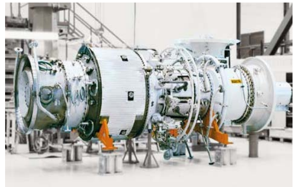
Fig 1. a) Draugen offshore platform, North Sea, Kristiansund, Norway. b) SGT-500 Siemens twin-spool industrial gas turbine.
