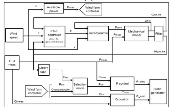
Figure 4: Aggregated Type IV wind turbine – source [6] & [7]
