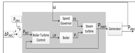
Figure 2: Aggregated CHP model – source [1] - [4]
