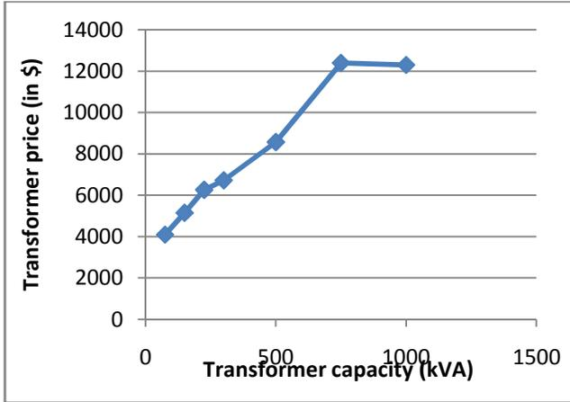
Figure 2 Distribution of transformer cost versus its capacity
