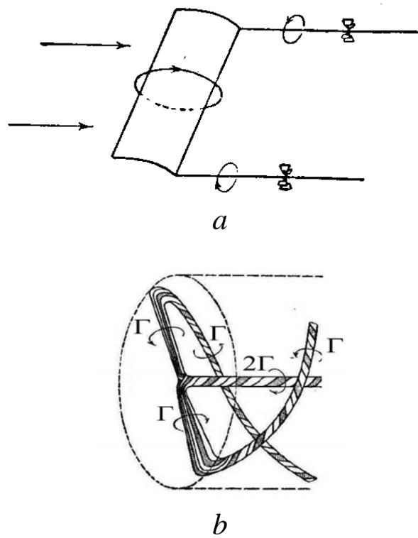
Fig.4 (a) the first elementary vortex model of a wing with a finite span based on a single horse-shoe vortex reported by Prandtl at the Gottingen congress in 1913;
