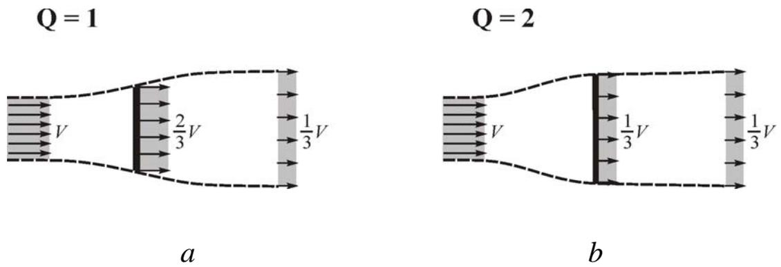
Fig.3 (a) Correct model of the Froude's actuator disc;
