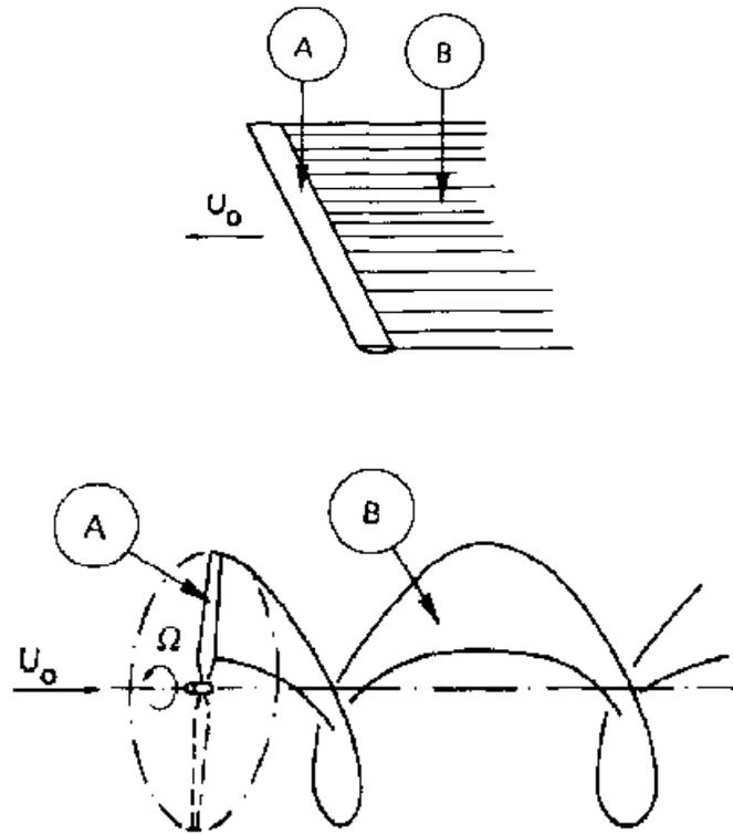
Fig.5 (a) Refined Prandtl's vortex model of a wing with elliptic load distribution published in 1918 [13];
