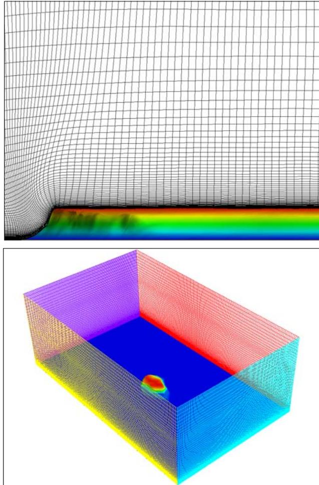
*Figure 6. Top: The volume grid is generated by marching the surface grid in the vertical direction using HypGrid3D. Bottom: Overview of the computational domain*
