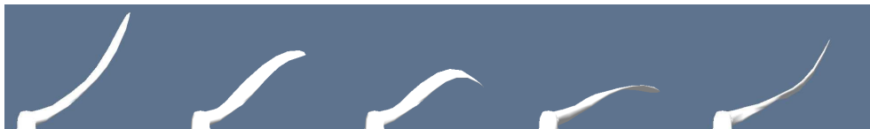
Figure 17. Frames from animation of an unstable blade flutter mode consisting of the second flapwise bending and first torsional blade modes. Animation from the isolated blade analysis performed by RISO with similar results as the ECN results in Figure 16.
