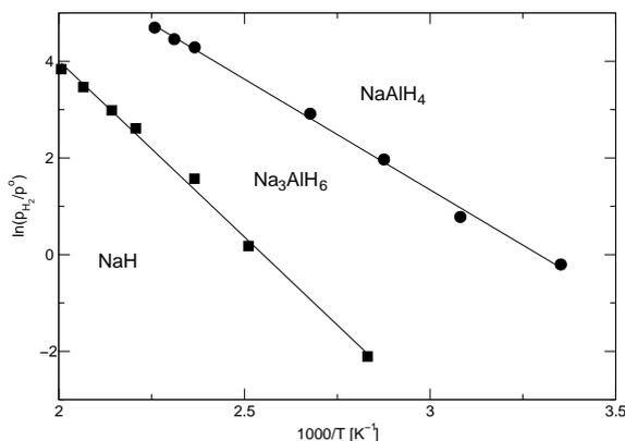
Figure 16. Van't Hoff plot for  $NaAlH_4$ . The stable hydride for each region of temperatures and pressures is marked on the graphic. Data points are taken from ref. [46].
