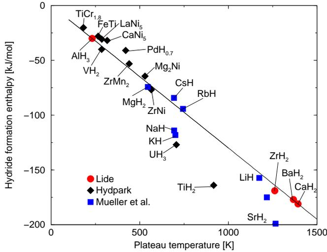
Figure 3. Hydride formation enthalpy,  $\Delta H_f$  per mole  $\text{H}_2$  as a function of the plateau temperature at 1 bar. The plateau temperature is calculated from reported thermodynamic parameters using the Van't Hoff equation. Data represented by circles is from ref. [11], data represented by squares is taken from ref. [12] and data represented by diamonds is taken from ref. [5].
