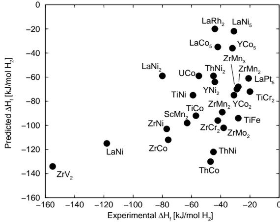
Figure 13. Predicted values of the formation enthalpy of intermetallic ternary hydrides obtained from Miedema model calculations [19] and the rule of reversed stability vs. experimental values [5, 15].
