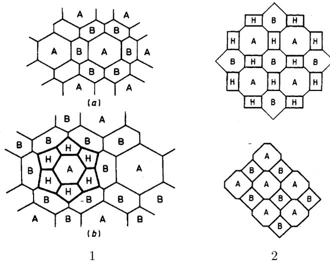
Figure 12. Schematic of the hydrogen positions in  $AB_n$  alloys. To the top left is shown an alloy poor in component A (hydride forming). Below is the corresponding hydride. To the lower right an  $AB$  ( $n=1$ ) type alloy rich in A is shown with its corresponding alloy (above). Adapted from ref. [19, 39].
