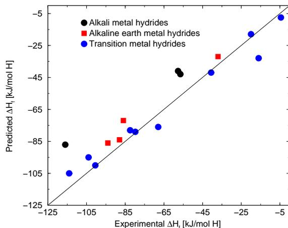
Figure 9. Predicted values of the formation enthalpy of binary metal hydrides obtained from DFT-GGA calculations [35] vs. experimental values from ref. [14, 11, 12, 15].
