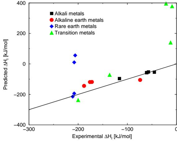
Figure 5. Predicted vs. experimental values for  $\Delta H_f$  calculated from the Born-Haber cycle. Experimental determined  $\Delta H_f$  for the alkali metal hydrides are from ref. [14], experimental  $\Delta H_f$  for the alkaline rare earth metal hydrides are from ref. [15], experimental  $\Delta H_f$  for the rare earth metal hydrides are from ref. [12] and experimental  $\Delta H_f$  for the transition metals are from ref. [11, 15]. The full line represents the case when pred. equal exp.
