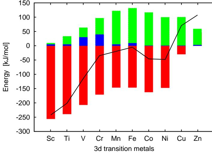
Figure 8. Trend in formation enthalpy for 3d transition metal dihydrides with the  $\text{CaF}_2$  structure (full line). The red bars represent  $E_{\text{hydride}}$ , blue bars represent  $E_{\text{transform}}$  and green bars represent  $E_{\text{expansion}}$ . All data points are adapted from ref. [34].
