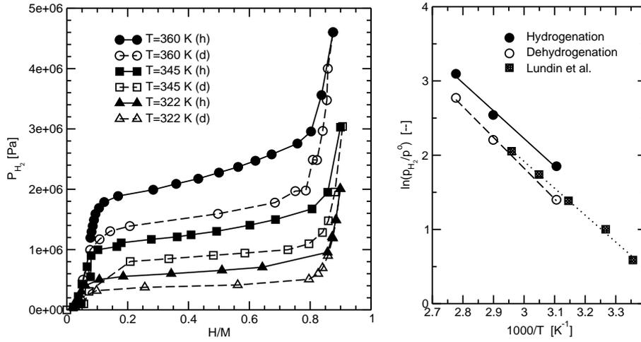
Figure 2. Left: Pressure-Composition-Isotherms (PCI) for  $\text{LaNi}_5$ . Right: Van't Hoff plot measured pressures at plateau midpoints ( $H/M=0.5$ ) from the PCI's. The Van't Hoff plot of Lundin et al. is from ref. [9]. PCI measurements were performed on a high pressure balance described in detail elsewhere [10].
