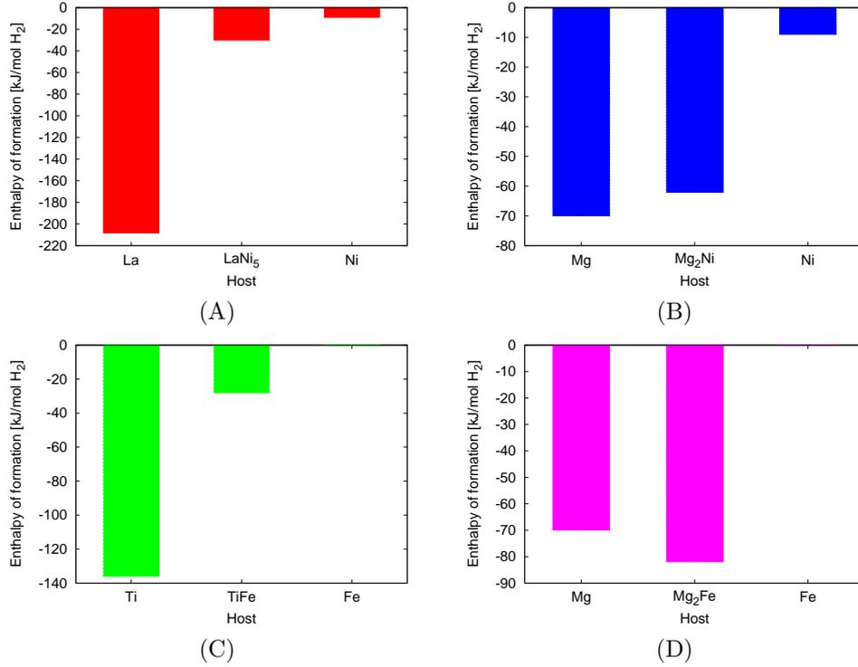
Figure 11. Enthalpy of formation of ternary hydrides and compared to their corresponding binary hydrides. A:  $\text{LaH}_2$ ,  $\text{LaNi}_5\text{H}_6$  and  $\text{NiH}$  [12, 5, 15], B:  $\text{MgH}_2$ ,  $\text{Mg}_2\text{NiH}_4$  and  $\text{NiH}$  [15, 36, 37], C:  $\text{TiH}_2$ ,  $\text{FeTiH}_2$  and  $\text{FeH}$  [38, 5, 15], D:  $\text{MgH}_2$ ,  $\text{Mg}_2\text{FeH}_6$  and  $\text{FeH}$  [15, 36, 37]
