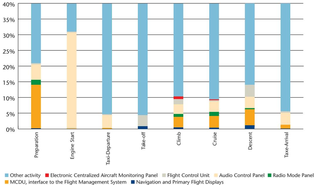
Figure 1: Human factors in aviation; what happens in the cockpit? The graph shows the time spent on manual activities for the "pilot flying" (PF). The data was collected during two real flights.
