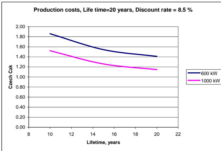
The calculated production costs for power generated by a 600 kW or a 1 GW wind turbine as a function of the expected economic lifetime of the turbines.
