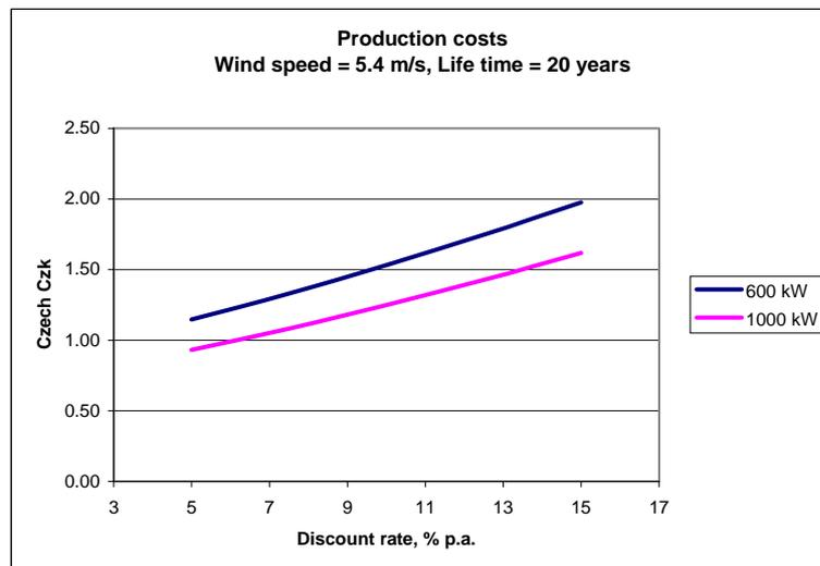
**The calculated production costs for power generated by a 600 kW or a 1 GW wind turbine as a function of the applied discount rate.**
