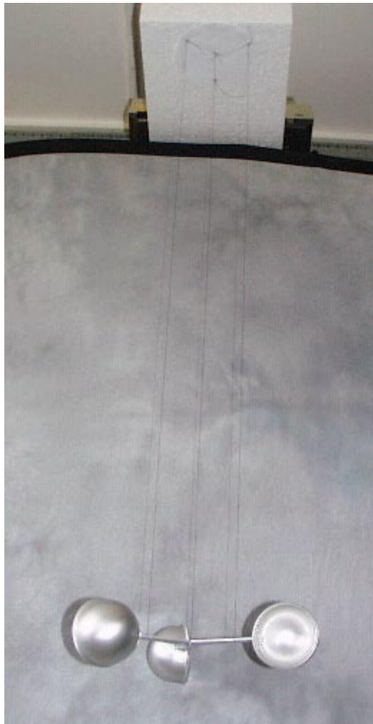
Figure 3-3 Determination of moment of inertia by oscillations of a Thies cup anemometer rotor
