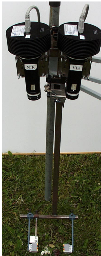
Figure 4: Picture of the LISS measuring devises. 2 SBIG CCD cameras equipped with a NIR and a VIS inspector imaging spectrograph, respectively and a Canon Digital IXUS located between these.
